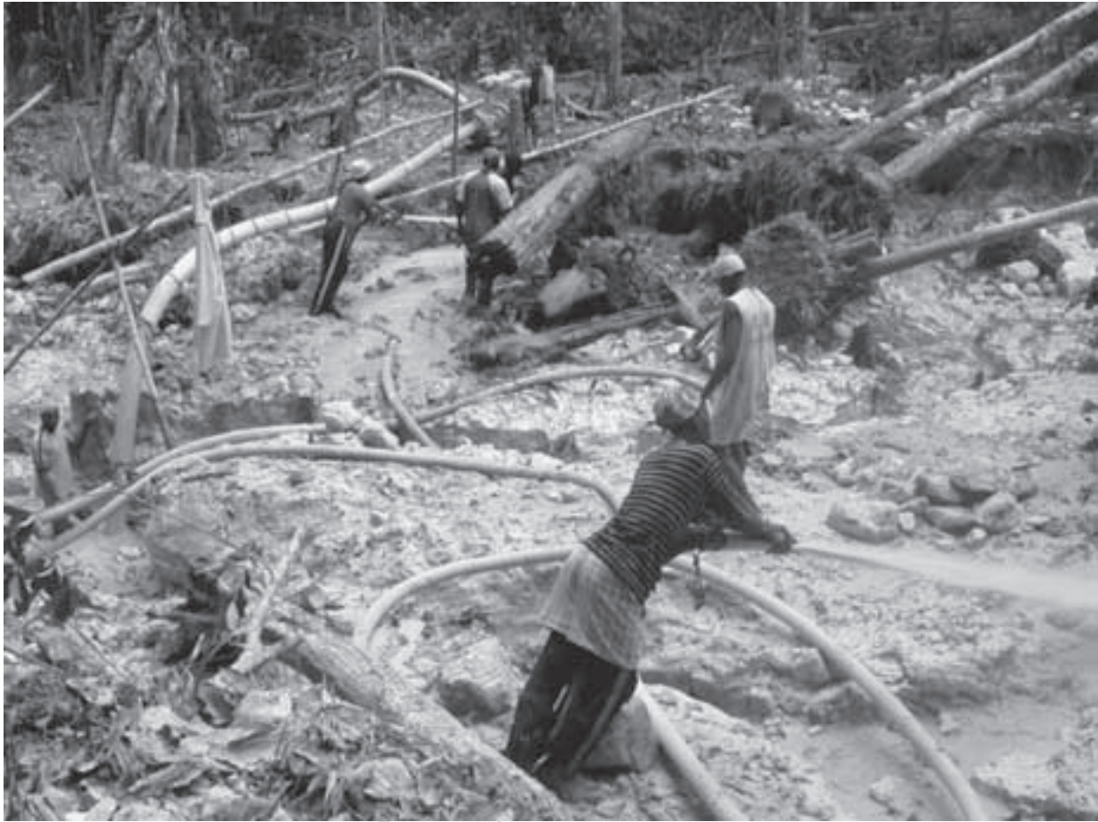
Plate 1. Small-scale mining pit. Two miners are operating power hoses to remove the soil (front and back-center). One miner stands next to the suction hose (left-center) to make sure that stones and branches do not enter and clog the hose. The two other miners remove waste materials from the pit. Hydraulic work at this site had started about one week before the picture was taken.
