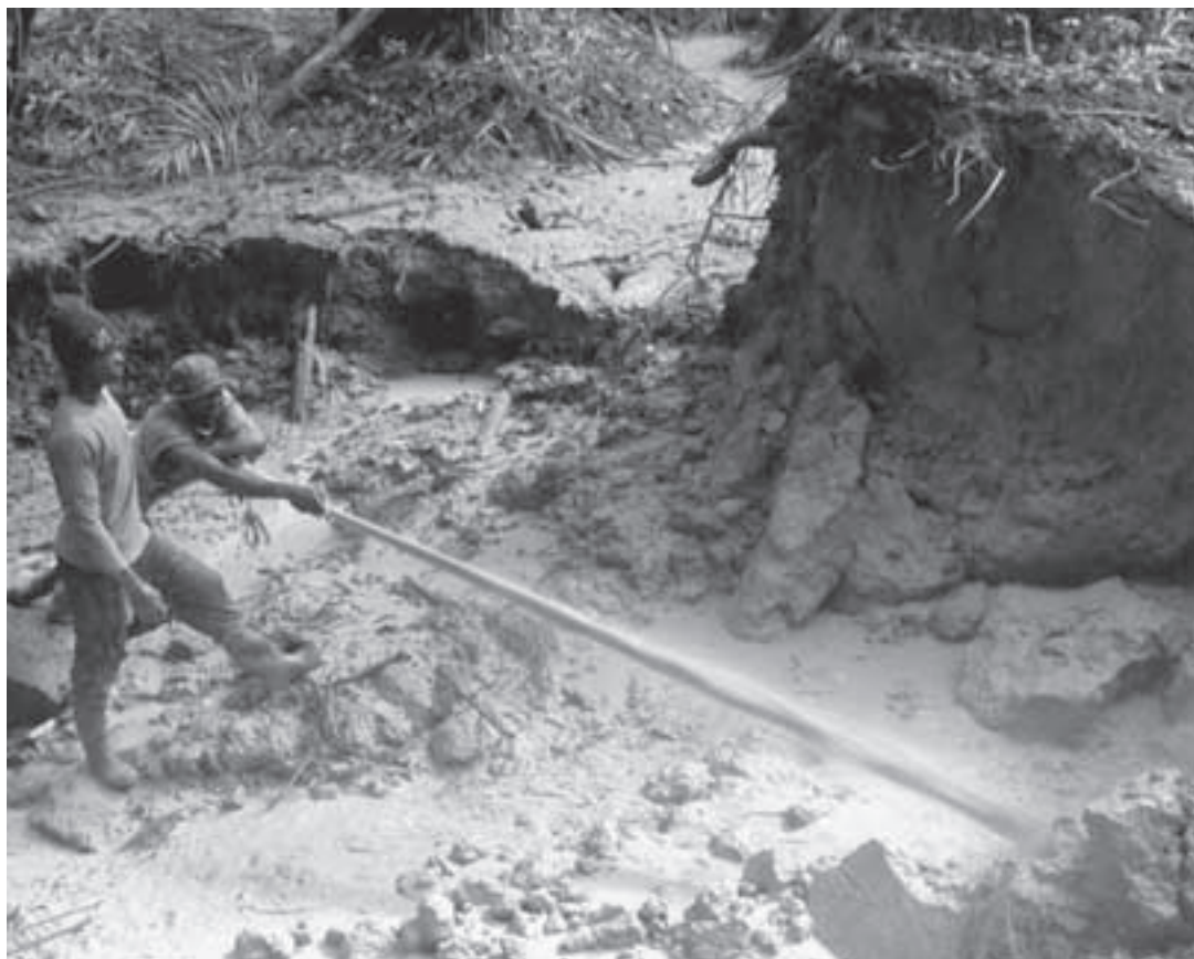
Plate 2. Miners use hydraulic power to remove the soil. The power of the water makes the miner lean forward on the hose.
